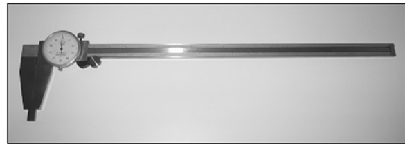
Figure 2. Dial caliper used for manual measurements of point-to-point distances.
